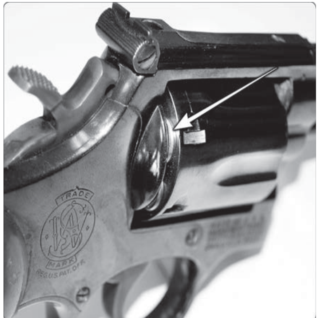
(Figure 6-2) Cylinder placement with partial load
